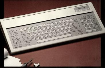
The Honeywell 84TC sealed touch panel PC-compatible keyboard is ideal for harsh environment applications and can be used with IBM PC, PC-XT, PC-AT and most compatibles.
