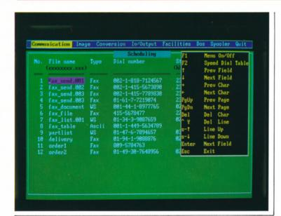
Message Scheduling-allows unattended message sending. SMARTFAX can be programmed in advance to broadcast a single message to multiple locations, and/or send multiple messages to multiple locations at different times to maximize the user's time and take advantage of discount phone rates.
